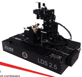
The Large Diameter Splicing System 2.5 (LDS 2.5) is an optical glass processing system designed for splicing, tapering, manufacturing of combiners, mode field adaptors, optical oscillators as well as other fused optical components. The LDS 2.5 is capable of performing splicing, tapering, scanning, cleaving, bundling diameters ranging from 125um up to 2.5mm.
